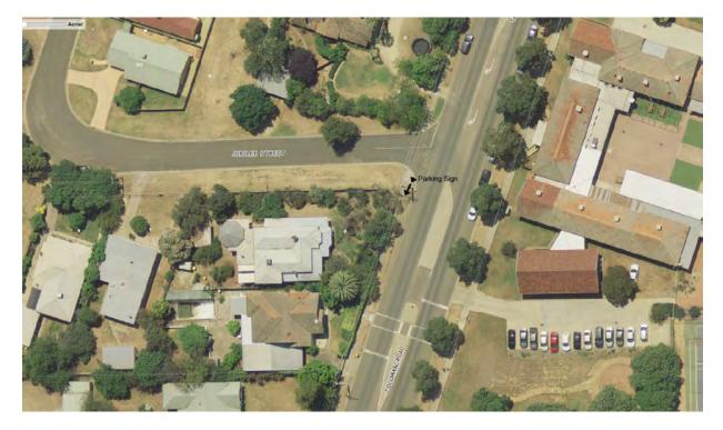
The parking sign on the south west corner of Tocumwal Road and Jubilee Street is quite close to the corner. This sign could be moved further away to prevent cars parking near the intersection. The car parking spaces could also be marked. This would provide additional sight distance at the expense of a car parking space, and would help those parking to see where parking was permitted.
