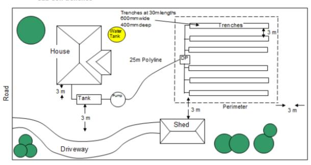
EXAMPLE 2 - Aerated waste water Treatment Plant and subsurface irrigation field layout
