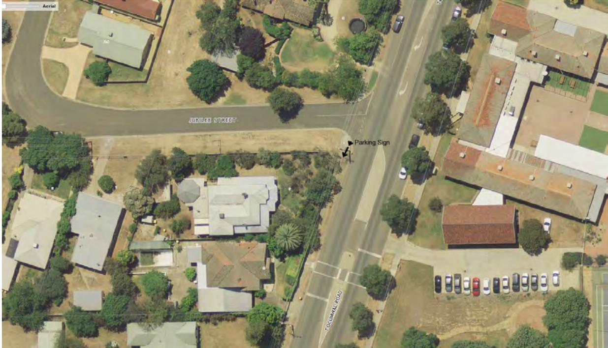
The parking sign on the south west corner of Tocumwal Road and Jubilee Street is quite close to the corner. This sign could be moved further away to prevent cars parking near the intersection. The car parking spaces could also be marked. This would provide additional sight distance at the expense of a car parking space, and would help those parking to see where parking was permitted.
