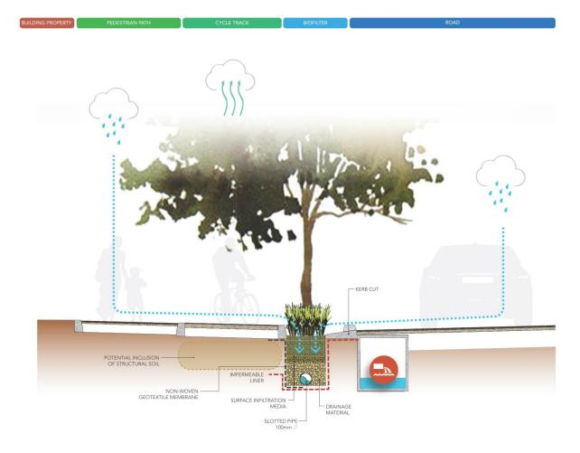
Figure 36. Passive tree irrigation cross section
