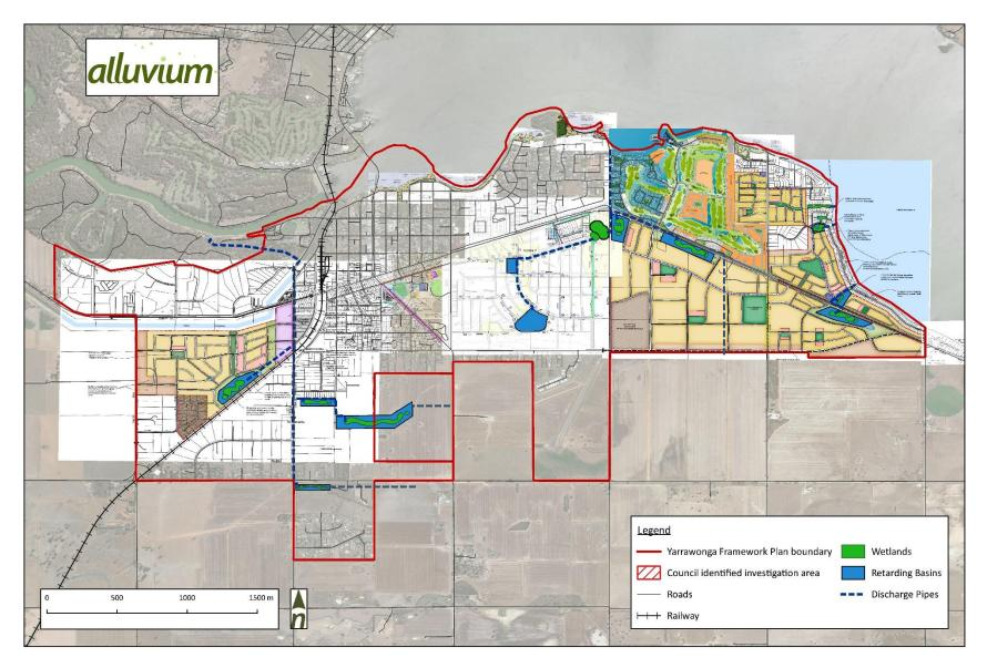
Figure 29. Proposed drainage asset placement – Option one overlaid on the developer plans
