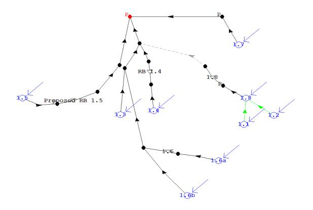
Figure 43 Yarrawonga West developed conditions RORB model
