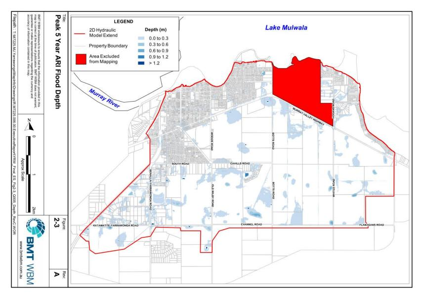
Figure 18. Peak 18% AEP Flood depth map for Yarrawonga (BMT WBM, 2015)
