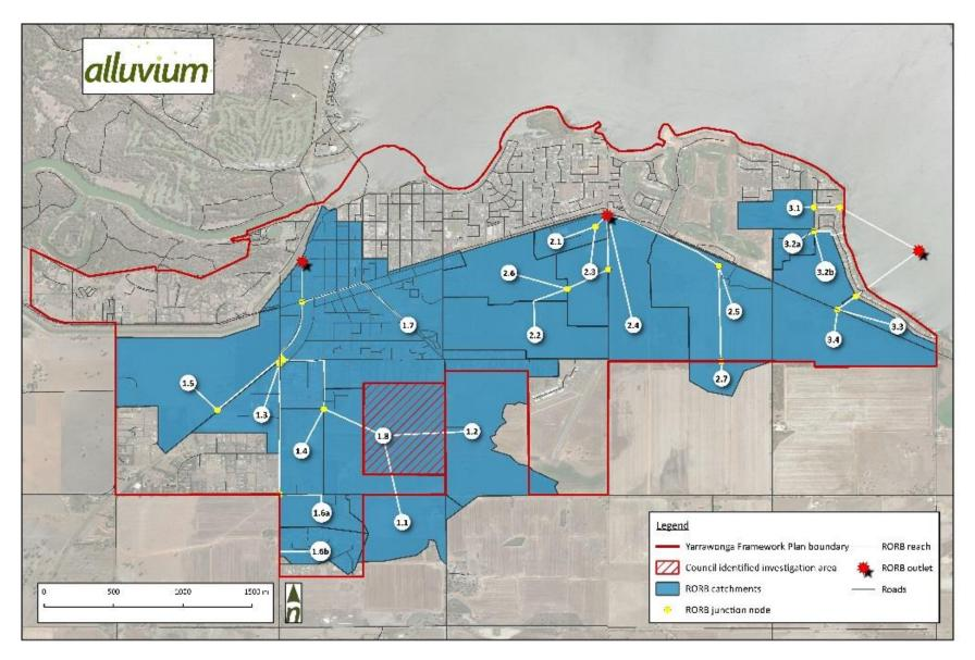
Figure 24. Yarrawonga growth area with RORB catchment breakdown
