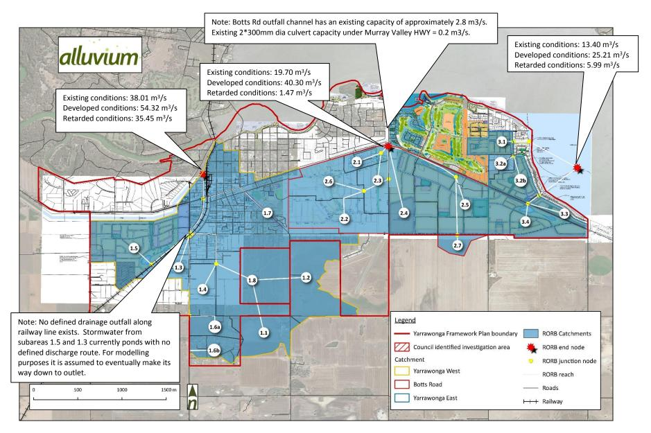
Figure 27. RORB delineation and flow retardation achieved for Option 1 – developed
