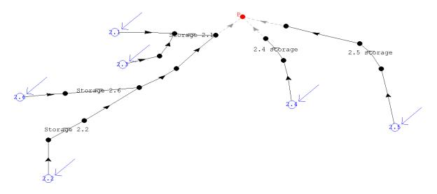
Figure 41. Botts Road developed conditions RORB model
