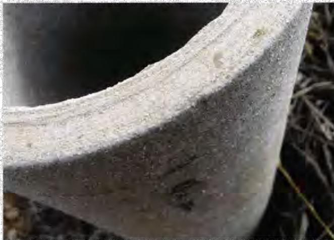
Photo 5 – Close up view of asbestos pipe, Lot 1.
